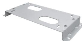
Raised foundation plate included. Height 34 mm. Floor fixing distance 353x117 mm, no. 4 Ø 11 mm, motor fixing distance 300x75 mm n.4 M8.
