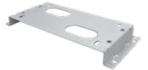
Raised foundation plate included. Height 34 mm. Floor fixing distance 353x117 mm, no. 4 Ø 11 mm, motor fixing distance 300x75 mm n.4 M8.
